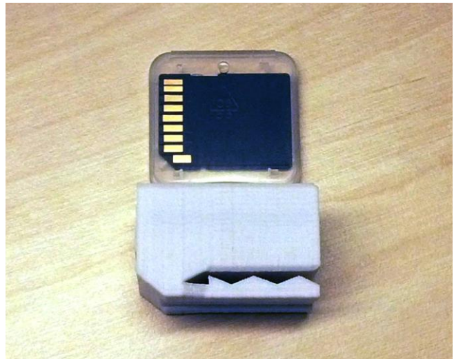
Figure 1. Side on view of pedestrian dead reckoning foot pod encapsulated in a 3D printed enclosure with outer dimensions 39 x 29 x 25 mm including clip for attaching to boot/shoe laces.
