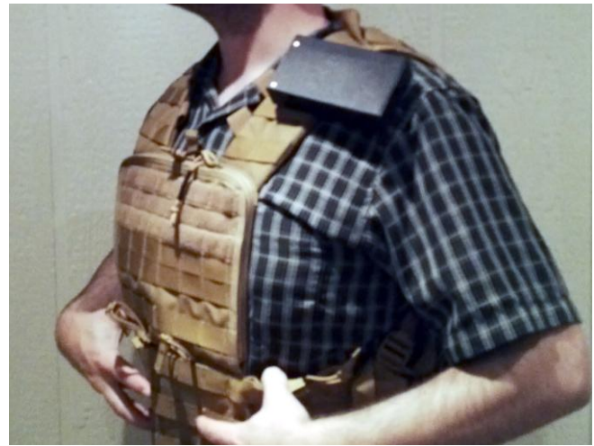
Figure 6. Main shoulder mounted system shown attached to a Modular Lightweight Load-carrying Equipment (MOLLE) vest via integral mounting clips in the enclosure. Outer enclosure dimensions are 13 x 7 x 3 cm.
