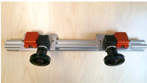
Figure 4: Visual navigation camera system. It is based on two identical modules comprised of a Point Grey Blackfly S 5.0 MP camera based on a Sony IMX250 monochrome sensor and an XSENS MTi-100 IMU. The modules are shown in a stereo configuration with 185° field of view Fisheye lenses.
