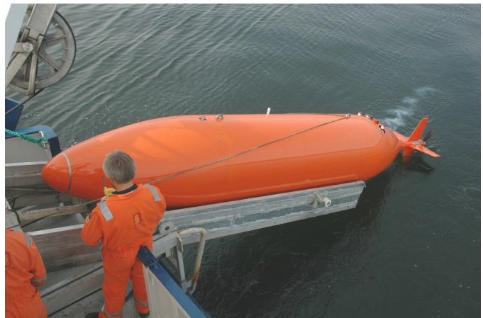
Figure 1. The HUGIN 4500 autonomous underwater vehicle during deployment for sea trials.
