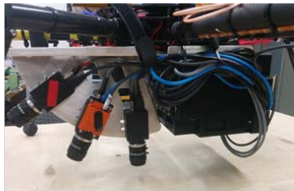
Figure 5. Onboard data collection system mounted under the Octocopter
