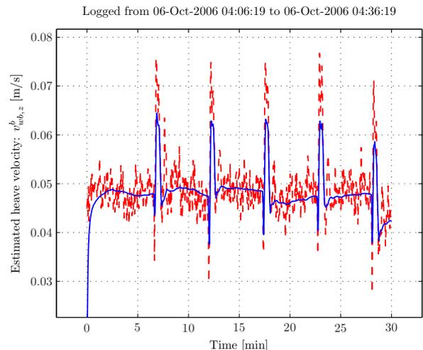
Fig. 6. Estimated vehicle water-relative heave velocity for square 3. The blue (solid) is the estimate of  $v_{wb,z}^b$  and the red (dashed) is the basis  $v_{eb,z}^b$ . From (4) it is straightforward to verify that  $v_{eb,z}^b$  and  $v_{wb,z}^b$  are approximately equal for zero vertical current and small roll and pitch angles.
