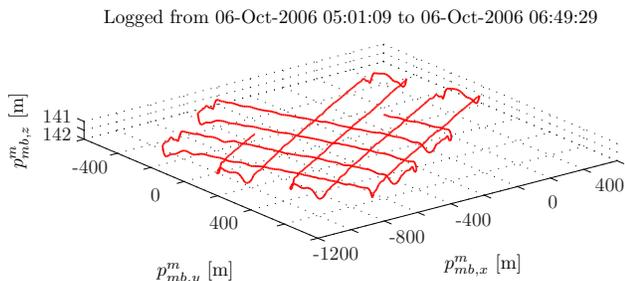
Fig. 5. Three dimensional vehicle lawn-mower trajectory. The trajectory shows the smoothed local position, which is considered as ground truth.
