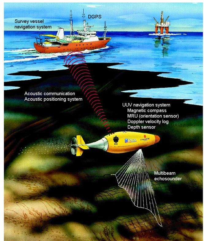
Fig. 1. A seabed mapping scenario with the HUGIN system
