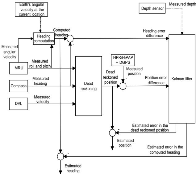
Fig. 2. Kalman filter structure
