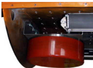
Figure 9 EM 3000 multibeam echo sounder transducer mounted on the HUGIN 1000 AUV.
