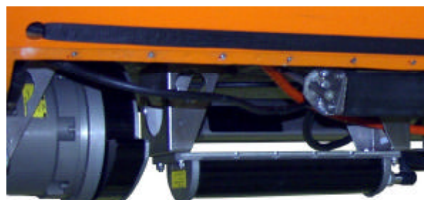
Figure 10 EM 2000 multibeam echo sounder transducers mounted on HUGIN 3000 AUV.
