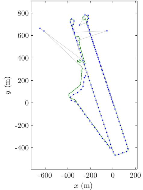
Fig. 2. Position measurements with outliers. Solid line shows the position estimate of the Kalman filter when no outlier filtering is performed.
