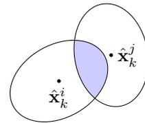
Fig. 6. Overlapping ellipsoid test. The covariance ellipsoids centered around the estimates should overlap if the estimates are statistically consistent.
