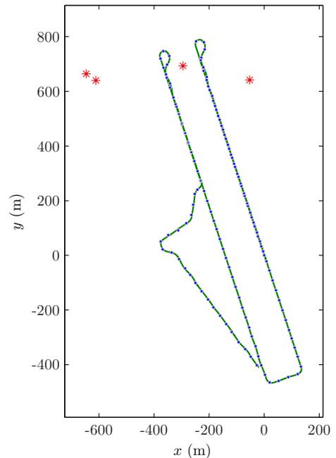
Fig. 3. Outlier filtered position measurements. Detected outliers are shown as stars. Solid line shows the position estimate of the Kalman filter when outliers are removed.
