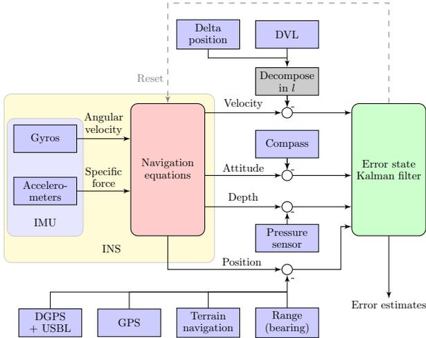
Fig. 1. Structure of an aided inertial navigation system (AINS) for underwater vehicles.
