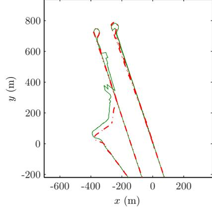
Fig. 5. Position estimates from two Kalman filters with different aiding sensors. Solid line is output from the filter with all aiding sensors. Dashed line is output from filter with no position aiding.
