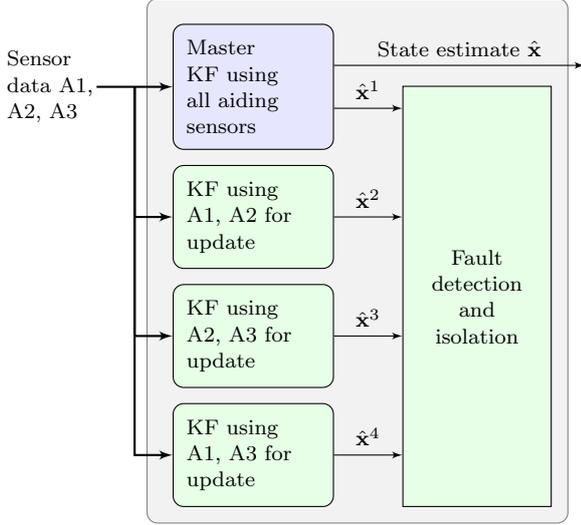
Fig. 4. A Bank of Kalman filters estimating the same state vector using different sets of aiding sensors.
